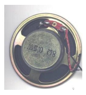
A *PC Speaker* is helpful as it could be used as a tool for diagnosing system hardware failures (different systems produce different beep sequences depending on the machine BIOS type).
