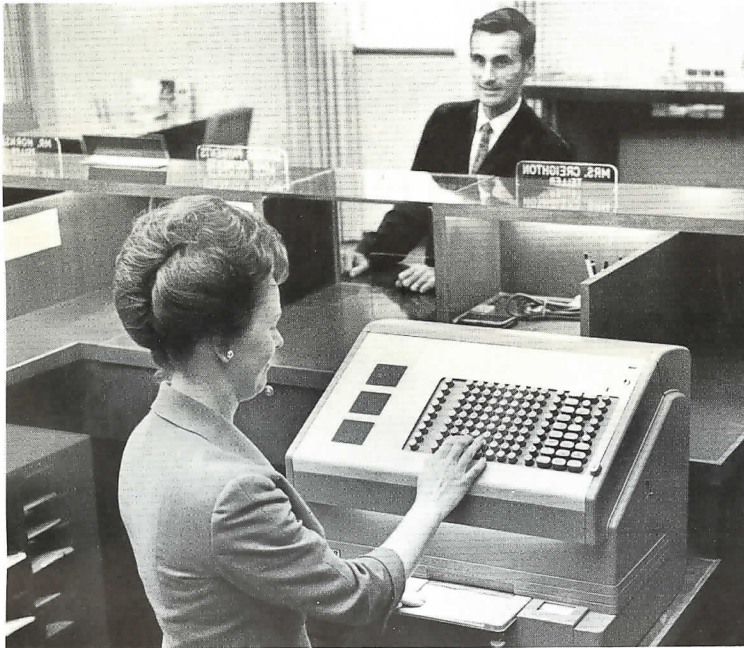
Teller sends data to computer miles away which processes transaction, activates teller's machine which updates depositor passbook.
