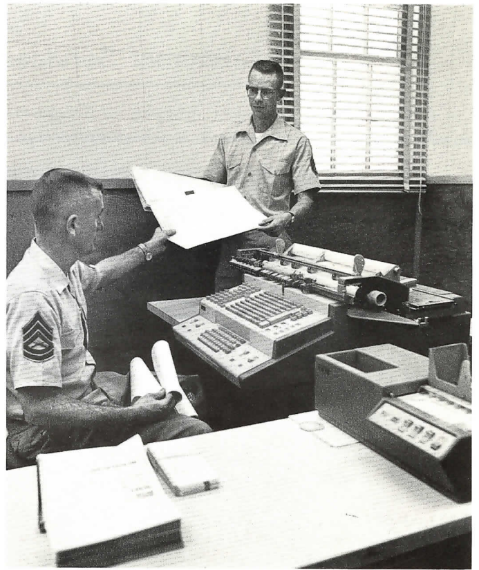
One of the first organizations to install NCR's new 395 electronic accounting system was a military base which is using the equipment for general accounting and for cost and statistical reporting. NCR punched card sorter, above, classifies data for input into system. Reports generated by this versatile equipment help officers achieve more efficient base operation.
