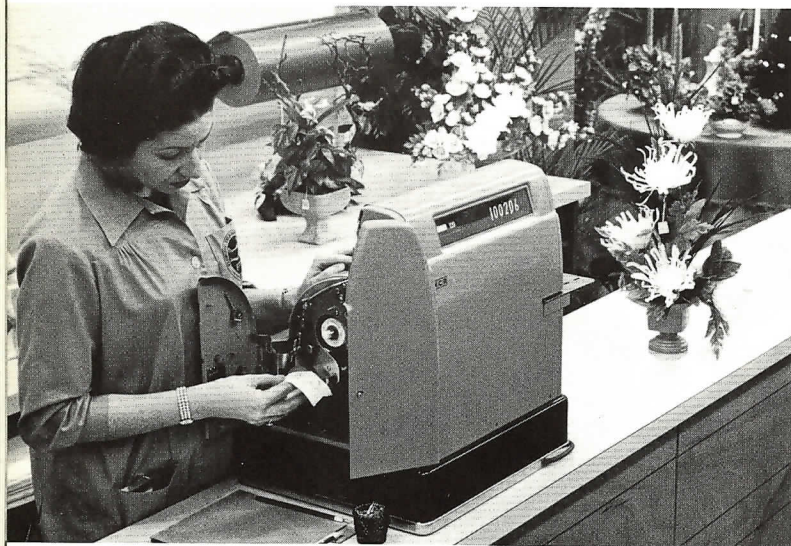
The services of NCR's larger data processing centers were augmented in 1964 by providing similar facilities at a number of branch offices. Above, an "optical" tape is removed from a florist's register. It will be sent to NCR office for processing.
