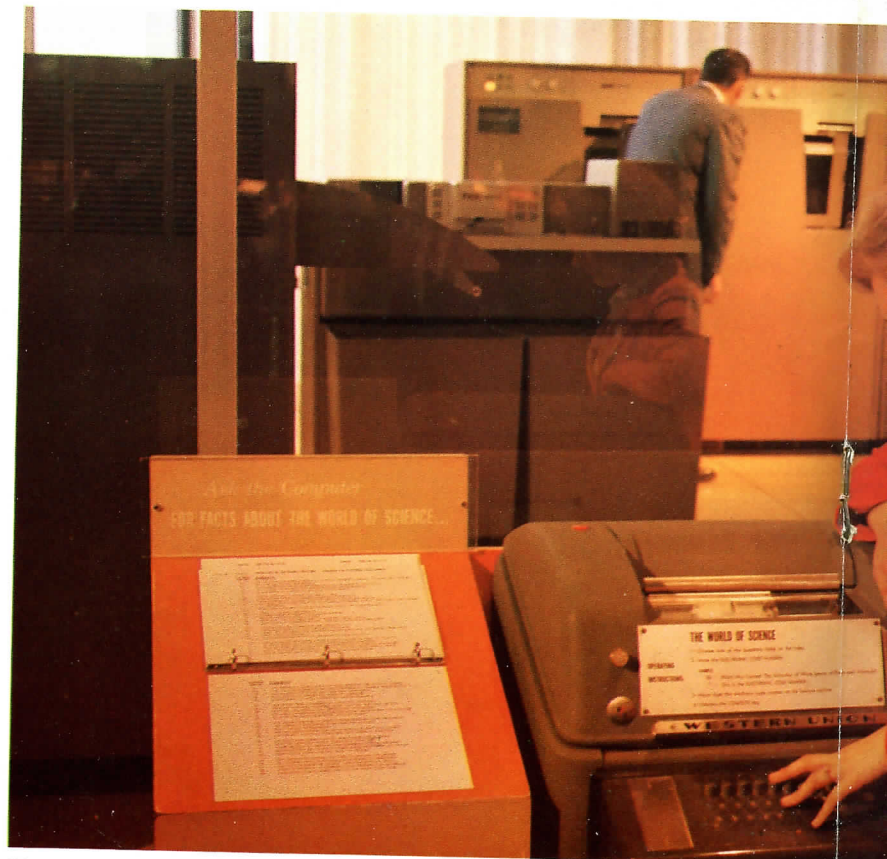
CRAM units of NCR 315 computer, background, can instantly locate facts from vast store of information in response to inquiries.
