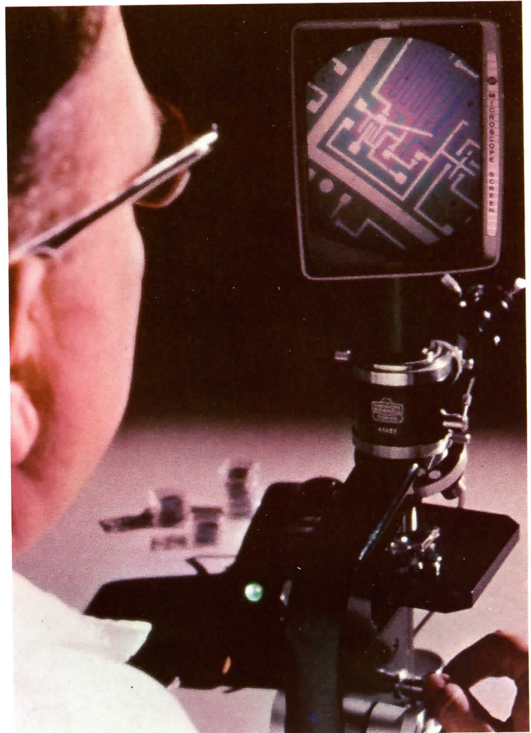
Hundreds of integrated circuits are formed on a one-inch chip and then inspected as shown in above laboratory photograph. Later they are cut apart and wired with hair-like strands of gold.
