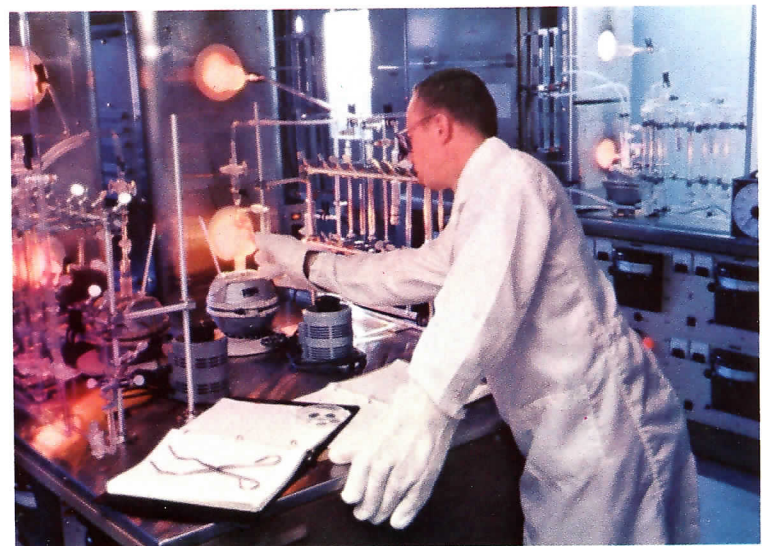
Electric furnaces in an NCR "clean room" are used to prepare integrated circuit base materials. The fabrication of integrated circuits requires a dust-free, carefully controlled atmosphere.
