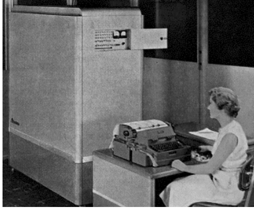
Figure 20. CRC102A computer and output printer. (Courtesy of the NCR Archive at the Montgomery County Historical Society.)
