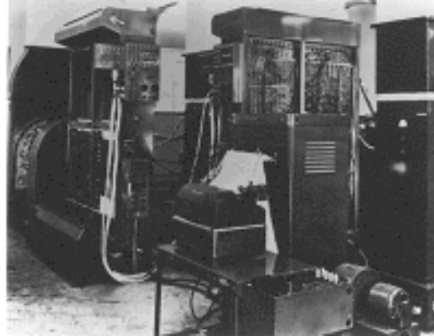
Figure 2. The Binac computer delivered in fulfillment of the contract to design an airborne digital computer. (Courtesy of the Computer History Museum, copyright 2003.)
