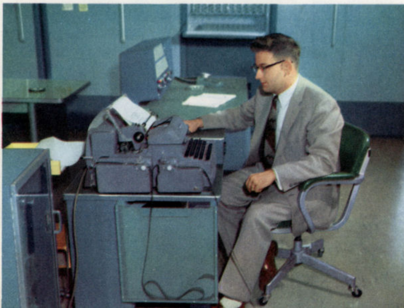
The results of the computer are typed out automatically on a special electric typewriter.
