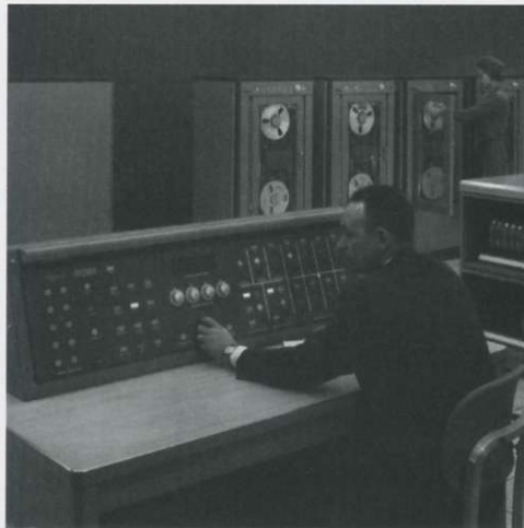
NCR 304, the first computer for NCR and first all-solid-state computer for business use.
