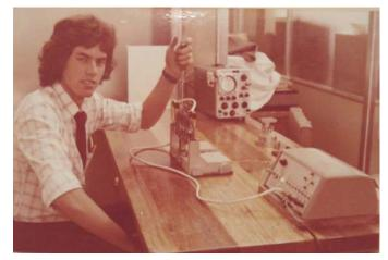
Hammer Module coils. The Hammer would strike a plate on which was mounted a sensor (I used a gramophone pickup).
