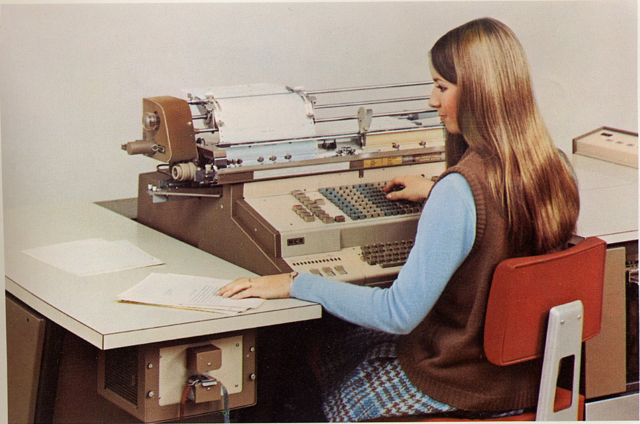
NCR 400 Electronic Accounting Machine is programmed by interchangeable loops of mylar tape
