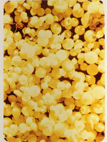
An encapsulated anticorrosion material
