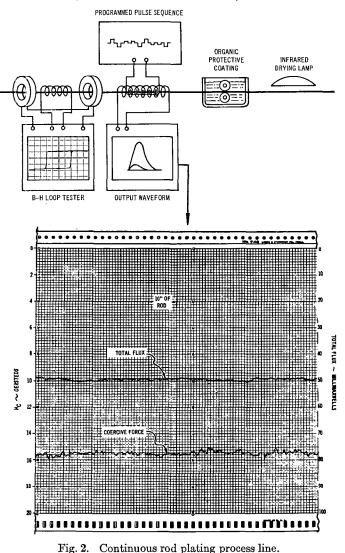
rig. 2. Continuous fou plating process line.
