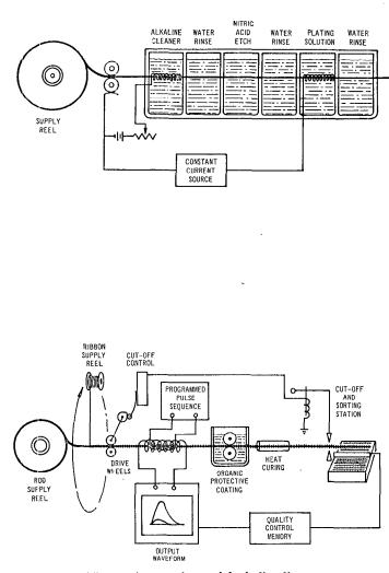
Fig. 3. Automatic coaxial winding line.
