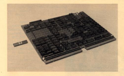
A comparison in size between a normal printed circuit board and the SCSI Chip (on the left). The chip is located in the center of the ceramic carrier with connector pins on the bottom.
