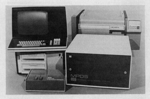
New microcomputer program development system from Process Computer Systems includes a PROM programmer, dual floppy disk system, high-speed line printer, CRT terminal, and interface modules plus software for \$12,000. Two lower-cost options are available for \$4900.
