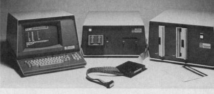
New development lab works with established microprocessors and will adapt to future ones, according to its manufacturer, Tektronix. Shown above are the 8002 lab (center), disk drive (right), and the CT-8100 video terminal (left) — one of several peripherals available. A companion model, the 8001, with in-circuit emulation only, has a ROM operating system rather than disk.
