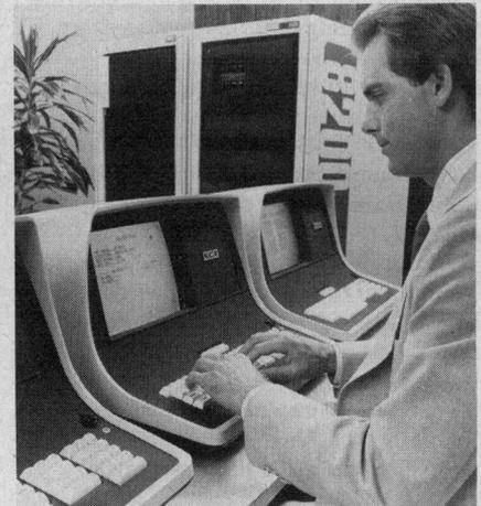
New interactive I-8270 system from NCR Corporation can accommodate from three to 24 visual display units.
