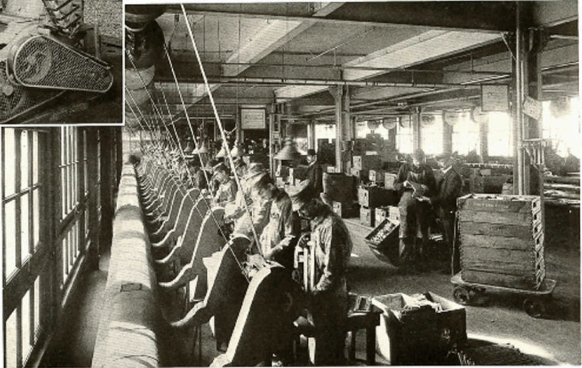
This factory was one of the first to install an automatic exhaust system to carry away metal and wood dust. This is just one of the ways in which work has been made healthful and safe
