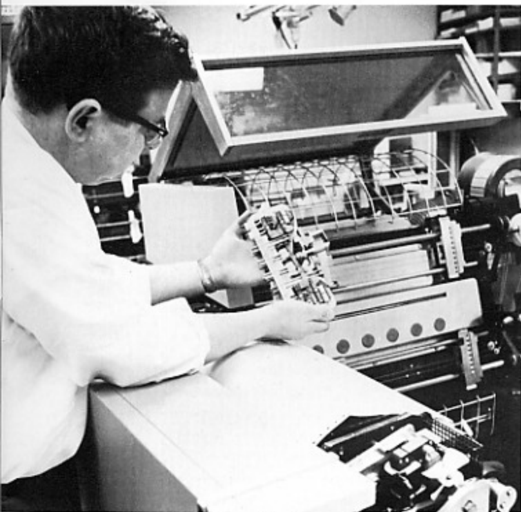
Jack Hiatt of Peripheral Equipment Engineering in Dayton examines hammer module that will enable Century Series printer to make sharp images on multiple copies.
