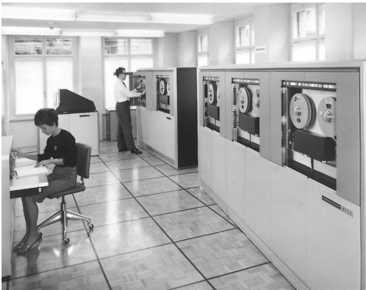
Figure 11. Bull Gamma 30 at SKA with magnetic tape units. (Source and copyright: Historical Archives Credit Suisse Group, Zürich.)
