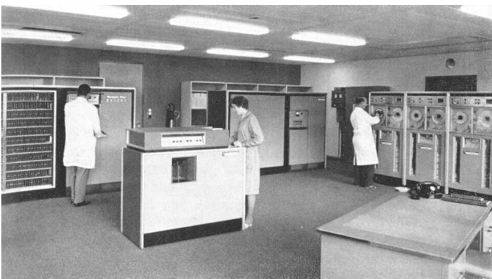
Figure 10. Univac UCT at SBG with magnetic tape units. (Source: SBG Blätter Juli 1965, p. 17, SBG, 1965. Copyright: Union Bank of Switzerland, Zürich.)
